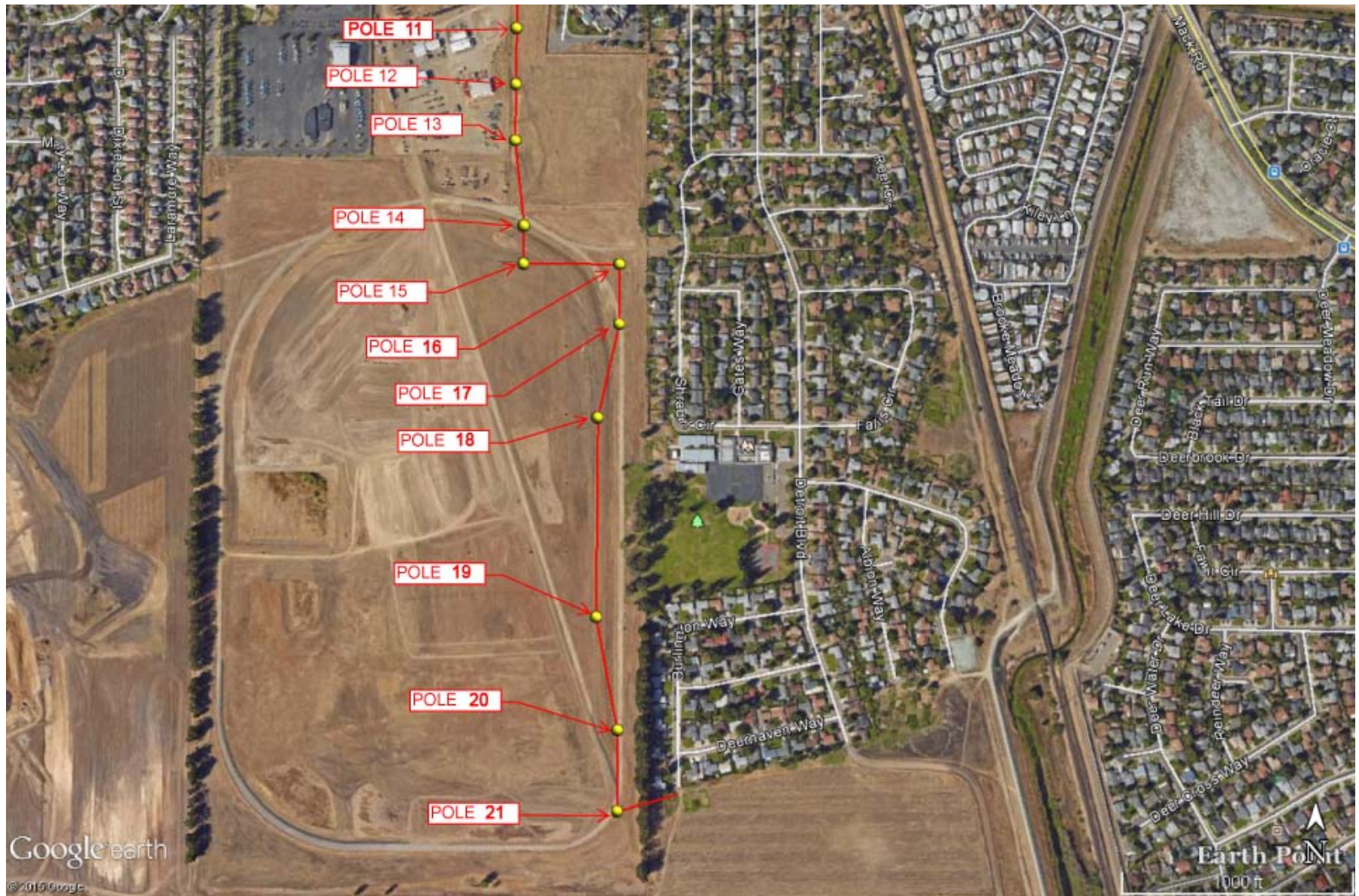
Figure 1-3b. 69KV Transmission Line Relocation – Southern Portion
